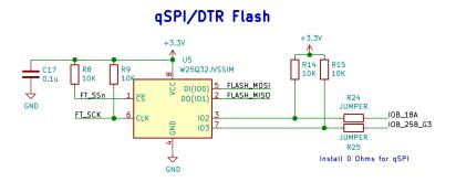
The corresponding portion of the layout is labelled qSPI for clarity and should be shorted as shown.
