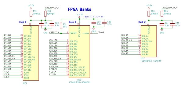
Bank 1 is connected to the 3.3V supply and cannot be modified since it is hooked up the the Flash and the FTDI parts, both of which are 3.3V devices.
