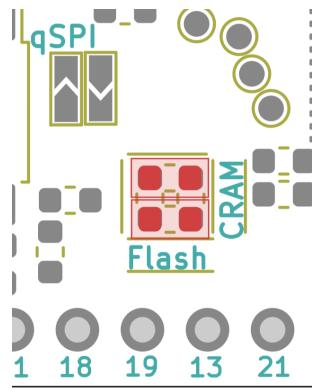
Removing R12/R13 and installing R11/R27 would look like the following layout:
