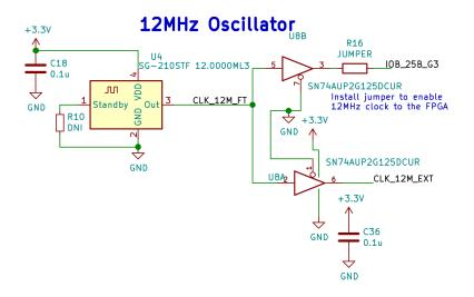
The 12MHz can be routed to the FPGA directly on the board to preserve signal quality and also to minimize external connection by shorting R16. Note that this marked as OSC on the silkscreen for clarity.
